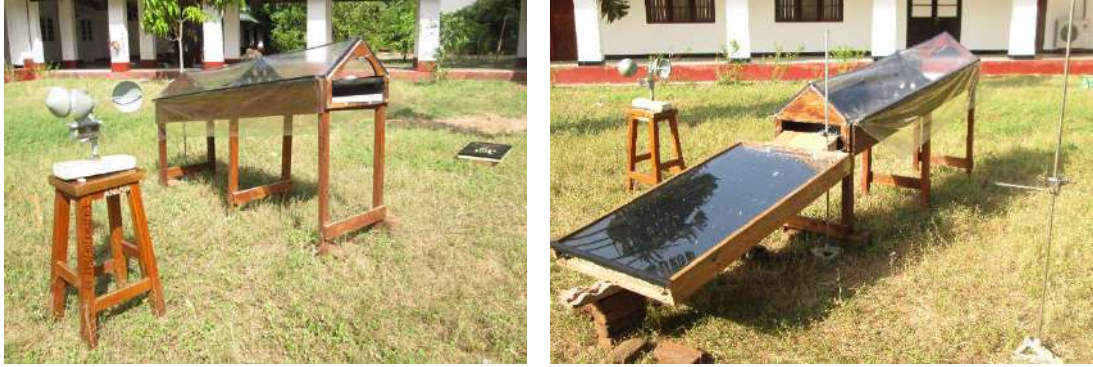
Figure 1: (a) The constructed solar tunnel dryer is in the field, and (b) when the auxiliary solar air heating unit is attached to the collector area of the solar tunnel dryer
