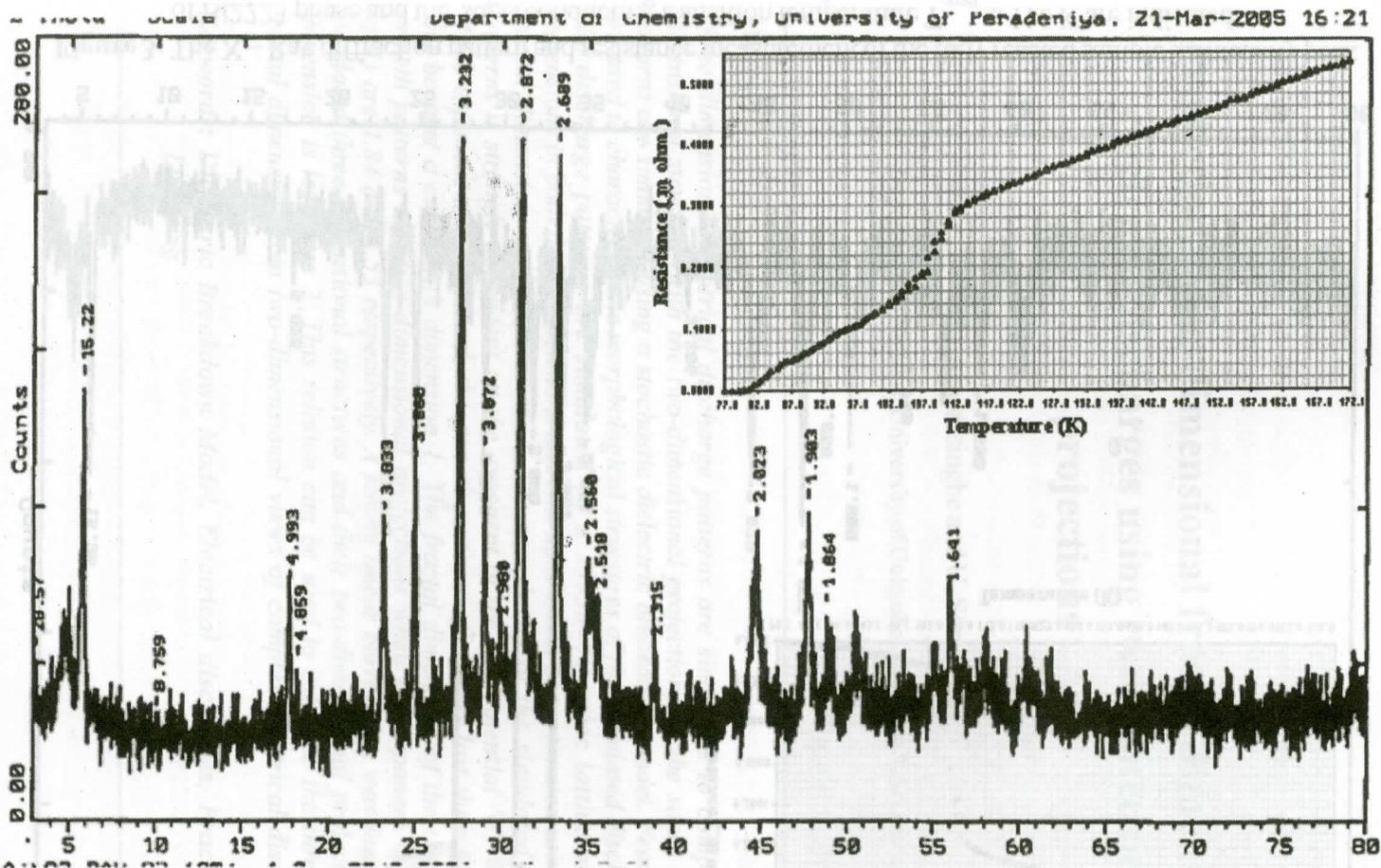
**Figure 2:** The X-Ray diffraction pattern and resistance measurement of the fully reacted sample 2. Intensity peak of Bi 2212 or Bi2223 phase and the superconducting transition temperature  $T_{\text{onset}}$  at 112 K are indicated.
